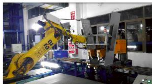
冰箱外壳折弯下料工作站 Robot unloading cell in the refrigerator casing bending site
